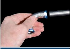
4. Assemble Fitting On Tube
