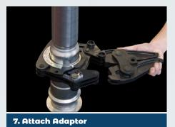
Squeeze the back of the adaptor arms together and hook onto the pressing collar.
