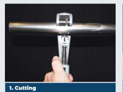
Cut the pipe using burr free approved cutters. Do not use oxyacetylene or abrasive cut off wheels. Pipes must be cut at right angles to their axis, using a pipe cutter or fine tooth saw, taking into account the depth of insertion into the fitting.
