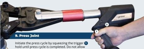
hold until press cycle is completed. Do not allow interruption to the press cycle. If the LED light comes on or warning beep sounds, the joint is NOT approved. If the hydraulic ram stops mid-cycle the automatic reset function can be manually over-ridden by depressing the reset button **2**. Any tool malfunction, check with our Technical dept.
